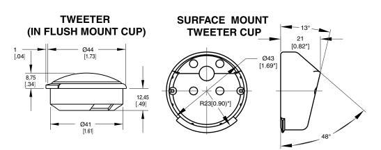
**M331i** General dimensions in millimeters and [inches]. Not to scale.
